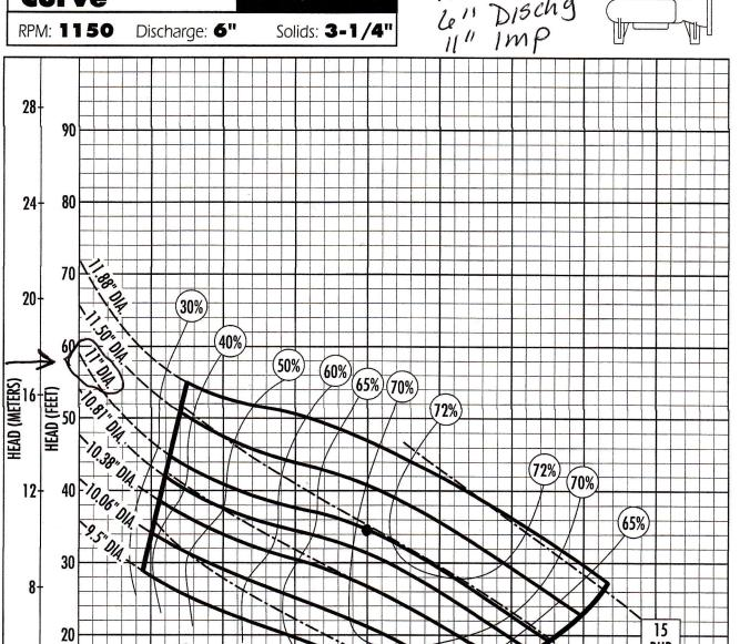
The curves reflect maximum performance characteristics without exceeding full load (Nameplate) horsepower. All pumps have a service factor of 1.2. Operation is recommended in the bounded area with operational point within the curve limit. Performance curves are based on actual tests with clear water at 70° F. and 1280 feet site elevation.
